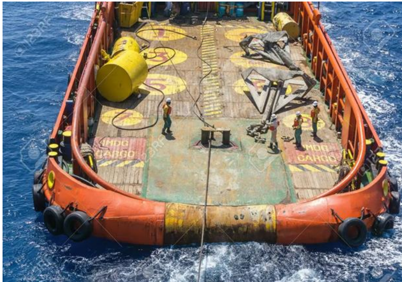
Figure 1. AHTS vessel running anchors (Source: https://www.shutterstock.com/ )
