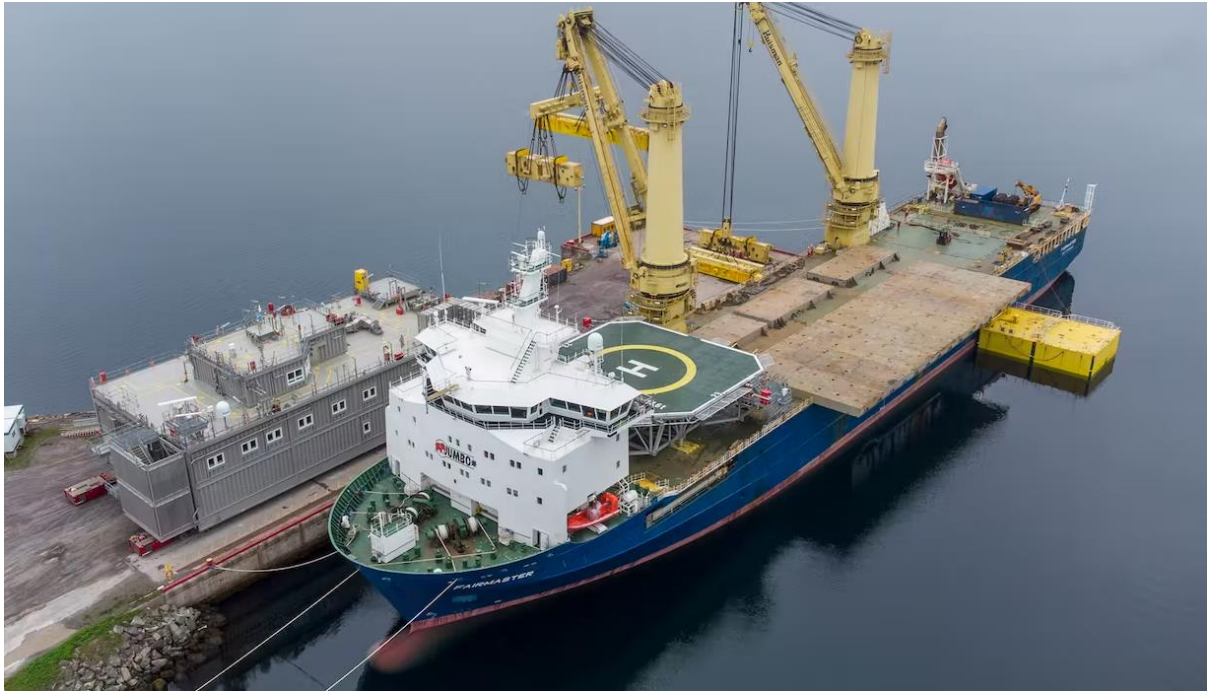
Figure 4. Stabilisation pontoons (Source: Jumbo maritime - Fairmaster, 2022)
