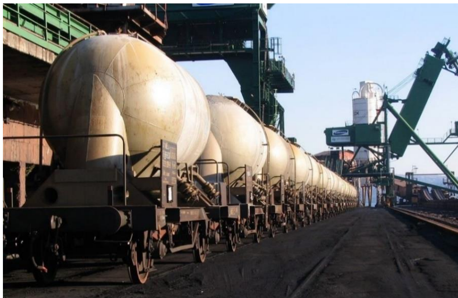
Figure 9. Terminal Bakar unloading UCK type of wagons (Source: CEMEX Croatia, 2022)
