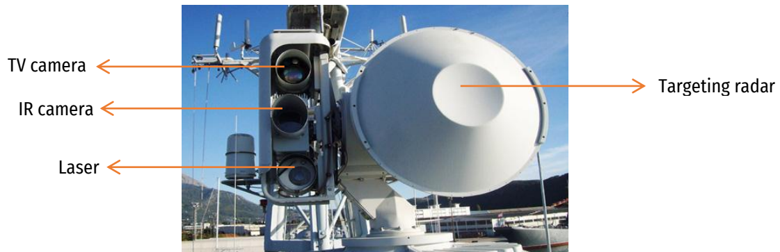
Figure 7. The director - a targeting radar, a TV camera, an IR camera, a laser (On Target Alignment, https://www.ontargetalignment.com )
