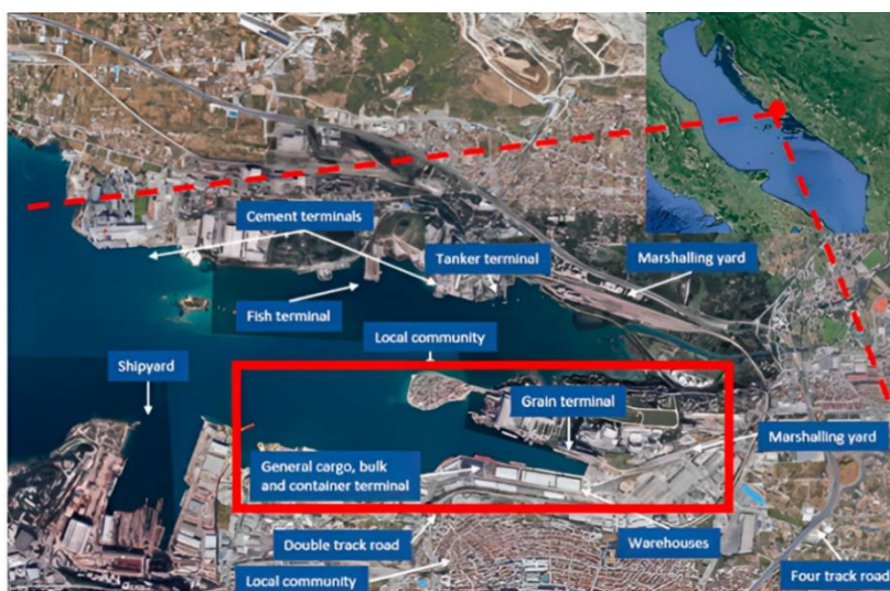
Figure 5. Location and overview of main functions of cargo terminals in the Port of Split (Vukić et al., 2022)
