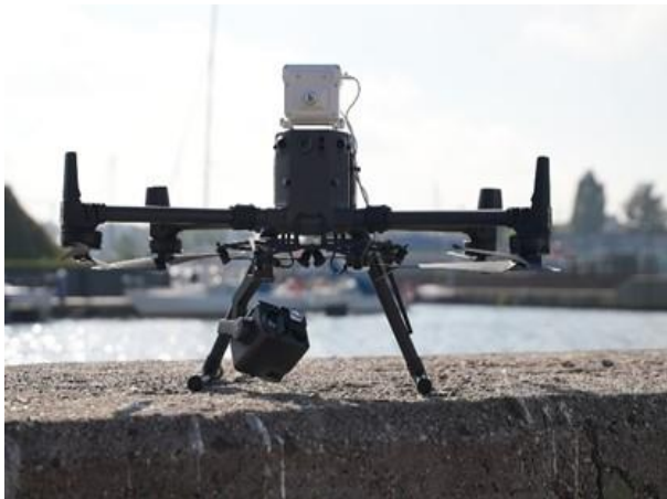
Figure 16. DJI Matrice 300 RTK drone with Sniffer 4D air pollution sensor and thermal imaging camera installed
