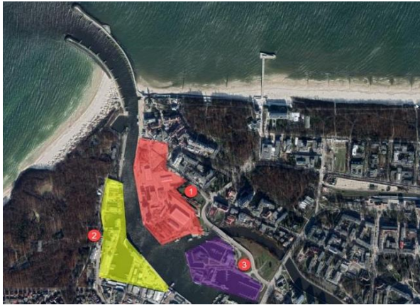
Figure 14. Port of Kołobrzeg. Layout. (1) – cargo handling and administration area, (2) – fishing port and shipyard area, (3) – yacht marina
