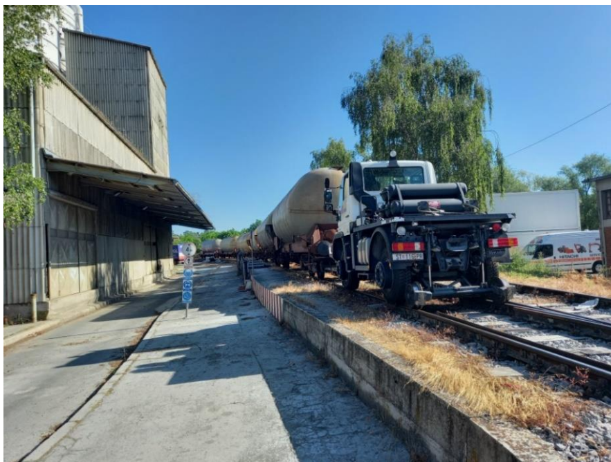
Figure 7. Terminal Maksimir - UNIMOG vehicle shunting the (Source: CEMEX Croatia, 2022)
