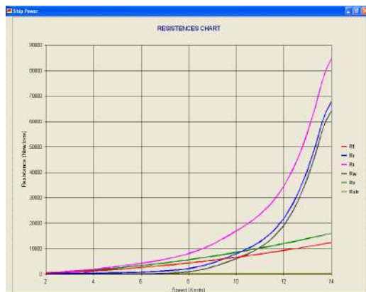
Figure 9. Graphical representation of resistance components, of the software “Ship Power V_1.0” versus the speed of ship.
