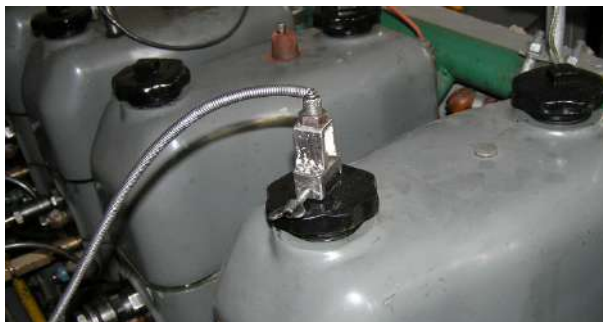
Figure 5. Vibration sensor mounted on cylinder head cover screw of SULZER 6AL20/24 type engine
