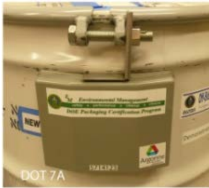
Figure 3. Sensor for a single-bolt mount
