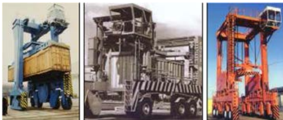
Figure 3. Straddler for vertical lifting and lowering of containers
