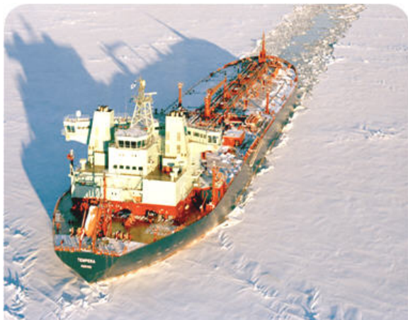
Figure 8. The aft part of the hull structure in double acting ships is composed of special reinforced with a double skin which breaks the ice when moving astern [37.]
