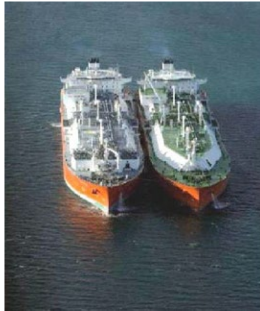
Figure 1. LNG transfer at open sea [6].
