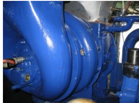
Figure 2. PBS Turbo PDH-35 type axial-flow turbocharger on SULZER main engine type 8AL25/30
