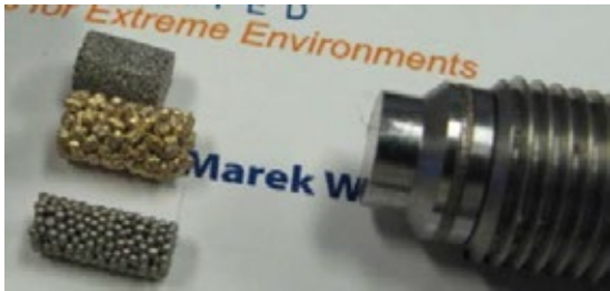
Figure 2. Examples of fire dampers for the Optrand sensors
