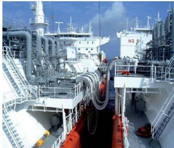
Figure 2. LNG transfer at open sea [6].
