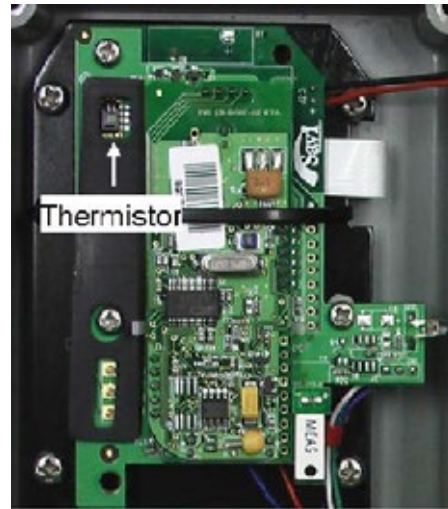
Figure 4. Thermostat built in a RFID tag
