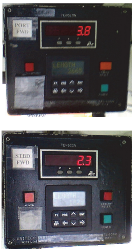
Figure 15. Tension and lineout meters for port and starboard bower anchor lines
