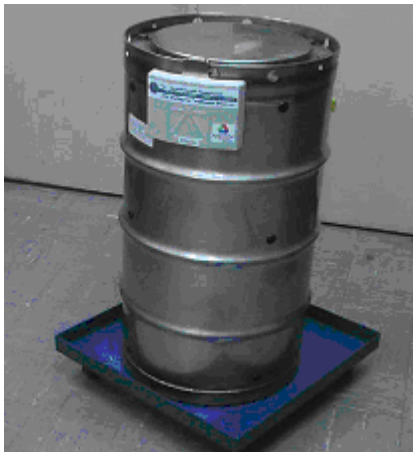
Figure 1. RFID tag attached to the drum type package of nuclear cargo
