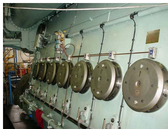
Figure 6. „Hoerbiger“ crankcase explosion relief valve on 2-stroke slow speed marine desel engine
