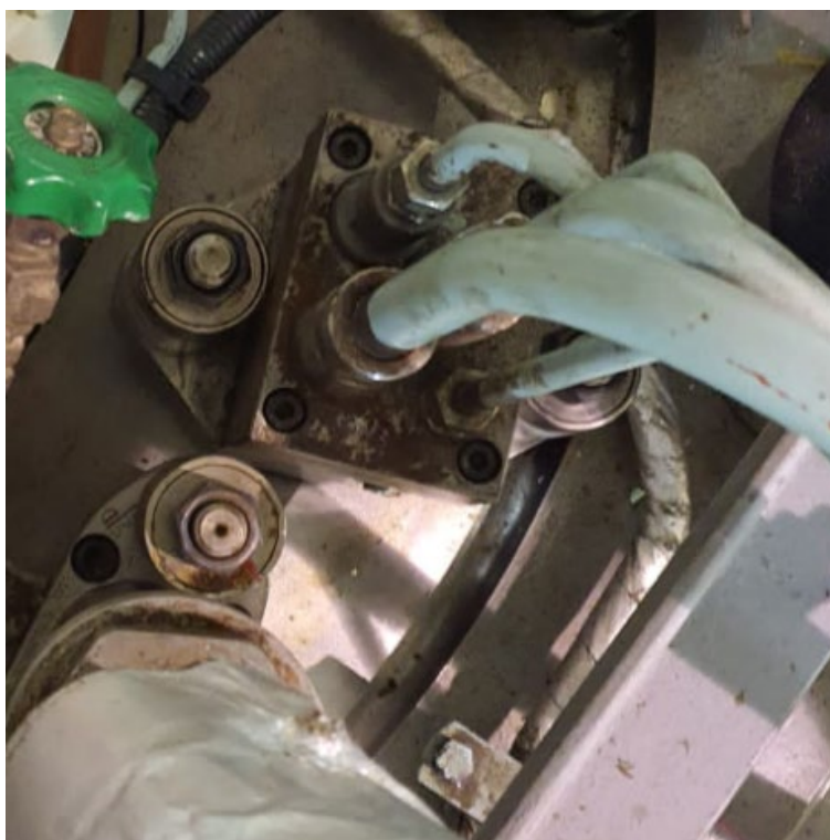
Figure 12. Fuel gas injection valve are mounted in the cylinder cover (Source: Authors, 2023)
