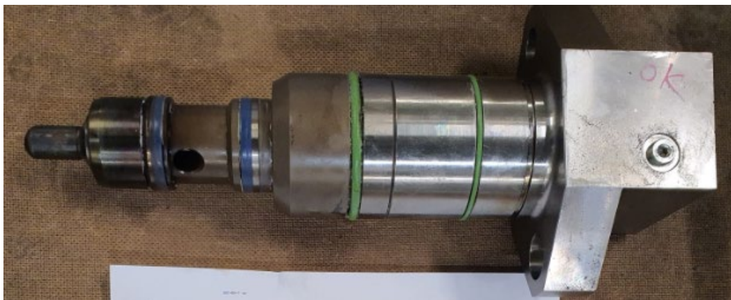
Figure 11. Fuel gas injection valve (Source: Authors, 2023)
