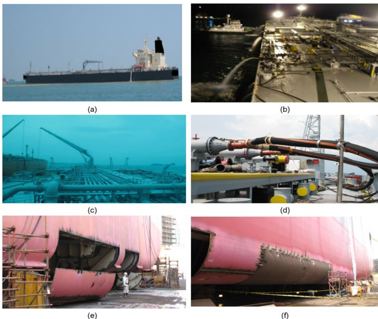
Figure 4. Aframax tanker: (a) Grounding position; (b) Salvage operation; (c) STS operation; (d) Discharging operation with portable hydraulic pumps; (e) Removal of damaged bottom plating (f) Renewal of bottom plating.
