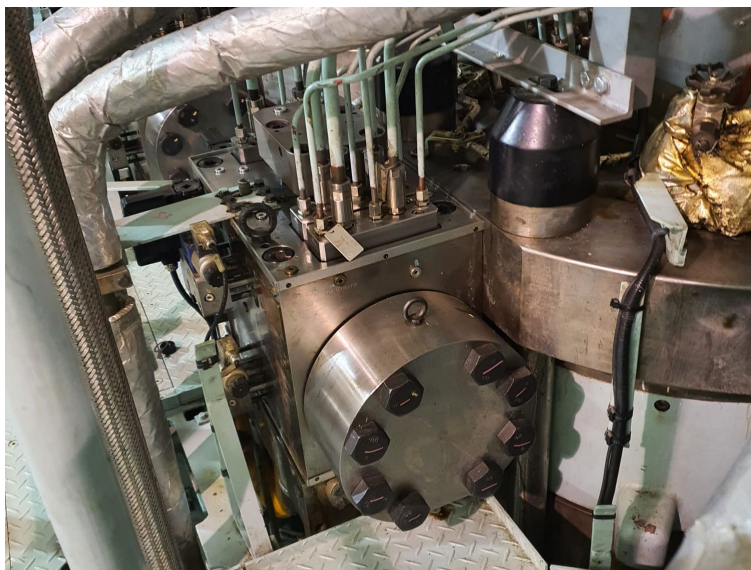
Figure 2. Fuel gas components (Source: Authors, 2023)
