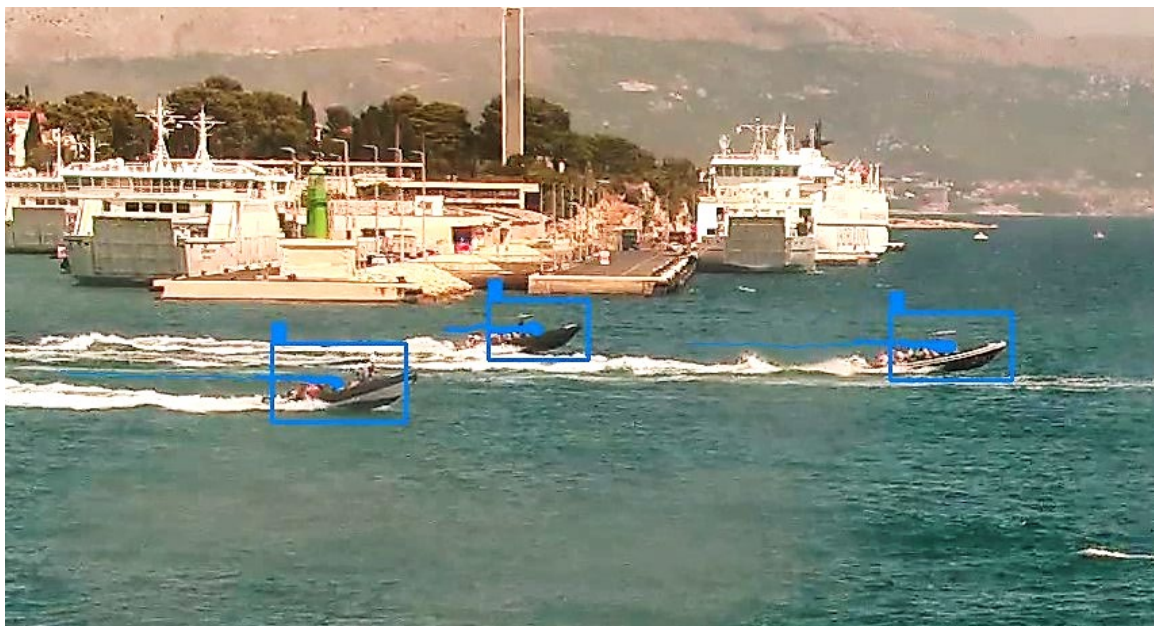
Figure 6. Camera stream with detected vessels
