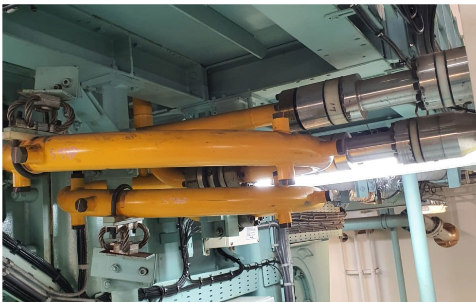
Figure 4. Helix pipe – compensator (Source: Authors, 2023)
